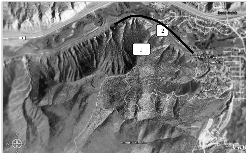
Figure 2-10: View of the West Gypsum Potential Site; 1-Aproxamate forebay location, 2- Afterbay may be located anywhere along the Eagle River I-70 corridor to facilitate siting. Eagle River I-70 corridor is marked in a bold black line.
